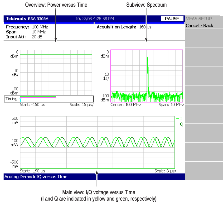
Figure 3–33: IQ versus time measurement
